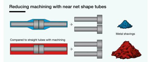
> Shaped tubes are metal cost effective with lighter and safer handling.
