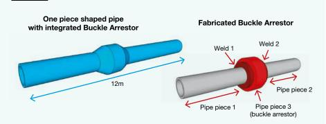
> Producing directly the final piece remove costly and hard to weld components.
