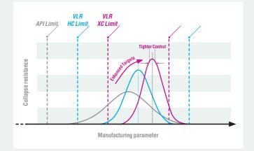
High Collapse grades are obtained by pushing the design parameters beyond standard API control. Additionally, eXtreme Collapse ratings are obtained by pushing the control of the production parameters beyond the targets defined for standard High Collapse grades.
