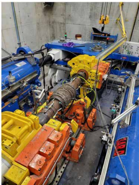
Figure 7—Load frame during hydrogen test protocol
