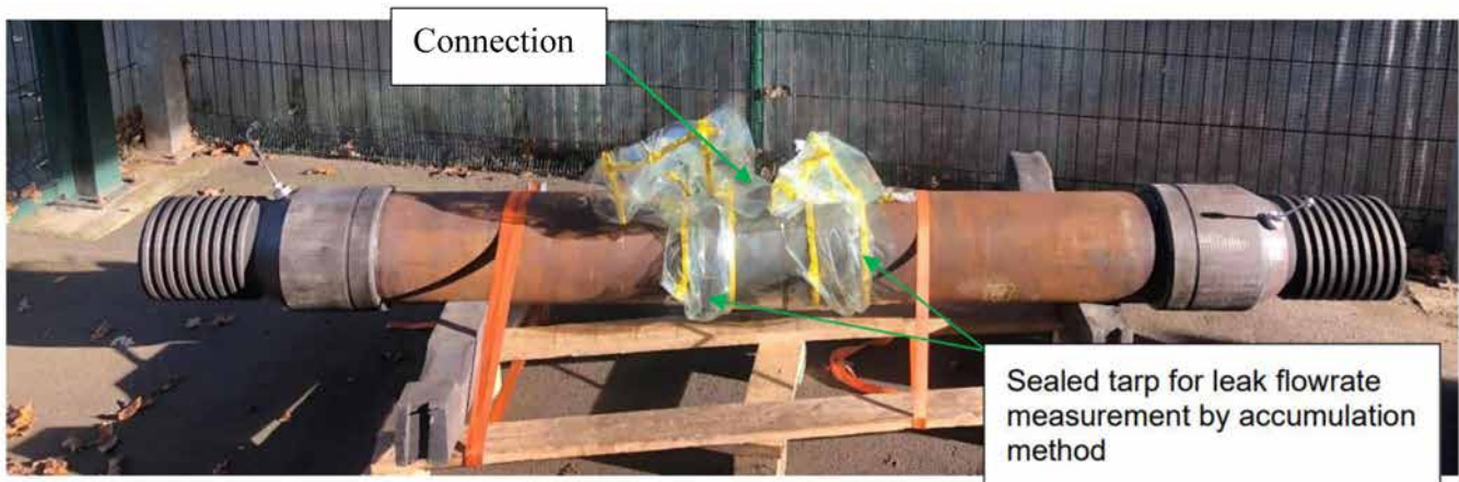
Figure 3—Test of the connection at 470 bars with leak detection by accumulation method
