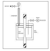
Figure 2: Test Equipment for Method A-NACE Standard Tensile Test
