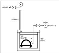
Figure 3: Test Equipment for Method C—NACE Standard C-Ring Test
