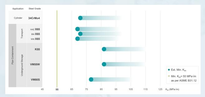
$K_1$  applied in the range of 134-176 MPa $\sqrt{m}$  was used during testing. The results of these evaluations demonstrated that all selected materials present a hydrogen stress intensity factor threshold  $K_{IH}$  greater than 67 to 87 MPa $\sqrt{m}$ , largely above the 55 MPa $\sqrt{m}$  minimum required by ASME B31.12.
