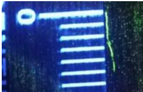
Figure 4: Example of surface defect revealed by MPI. These defects could be local cracks or lack of material after machining.
