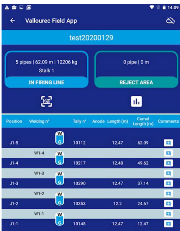
Figure 5. Best-Fit-Finder, Tag Tally screenshot: as-laid sequence of welded pipes is recorded, with each joint and weld being identified.
