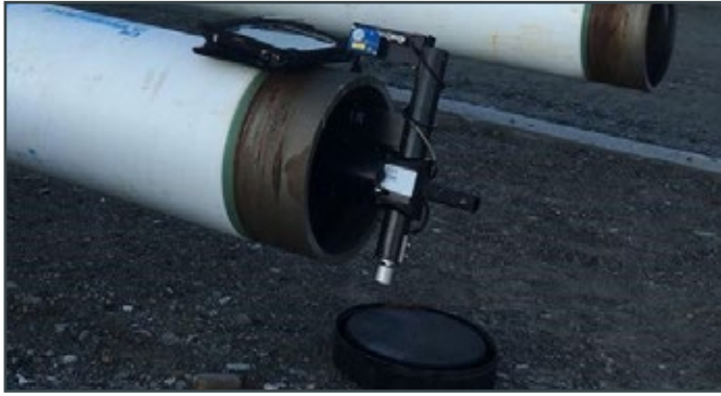
Figure 2: Portable Pipe End Measurement Tool
