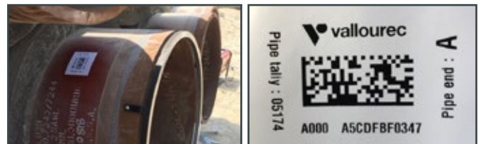
Figure 1: Data Matrix tags ensuring unique pipe end identification
