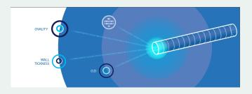
During product design phase, acceptable target ranges are set for these parameters based on the Vallourec Collapse Proprietary model, and then controlled during production: the tighter such control becomes, the higher the outcome collapse rating.
