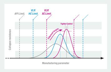
High Collapse grades are obtained by pushing the design parameters beyond standard API control. Additionally, eXtreme Collapse ratings are obtained by pushing the control of the production parameters beyond the targets defined for standard High Collapse grades.
