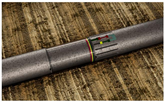
Monitoring mandrel deployed on casing with its sensor, battery module, and transmitting coil. (*Courtesy Vallourec*)
