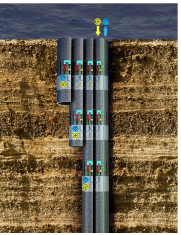
This is a co-development with OpenField Technology, which supplies the miniature sensors that are embedded outside of the pipes to capture and steadily stream data concerning temperature and pressure, ensuring that the pipes function correctly and maintain their structural integrity.
